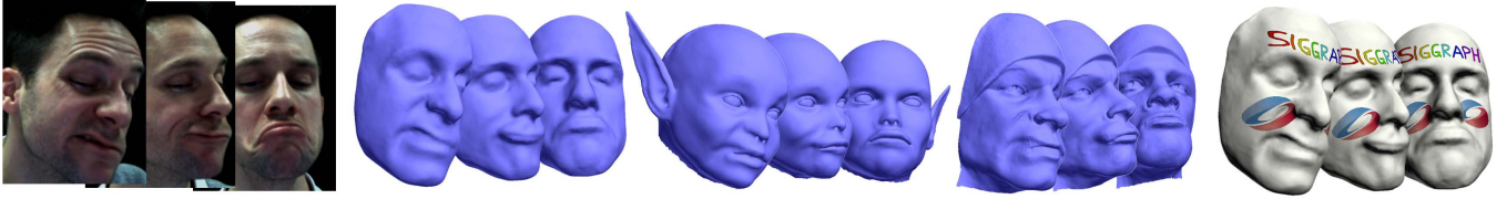
Figure 7: Applications for live non-rigid capture. Left: detailed facial expressions are re-targeted. Right: spatio-temporal coherent re-texturing of template meshes for the same input sequence.
